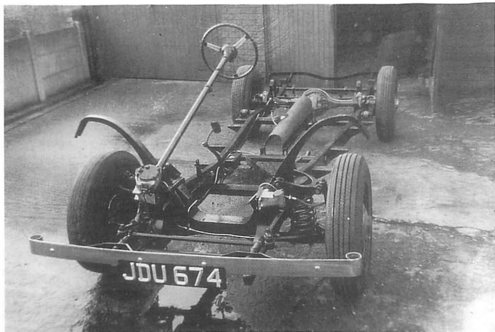
A TA 14 chassis converted to coil spring front suspension. This photograph of the chassis shows the details of the conversion, including a unique steering idler box and a slimmer cross-member than the production version.
