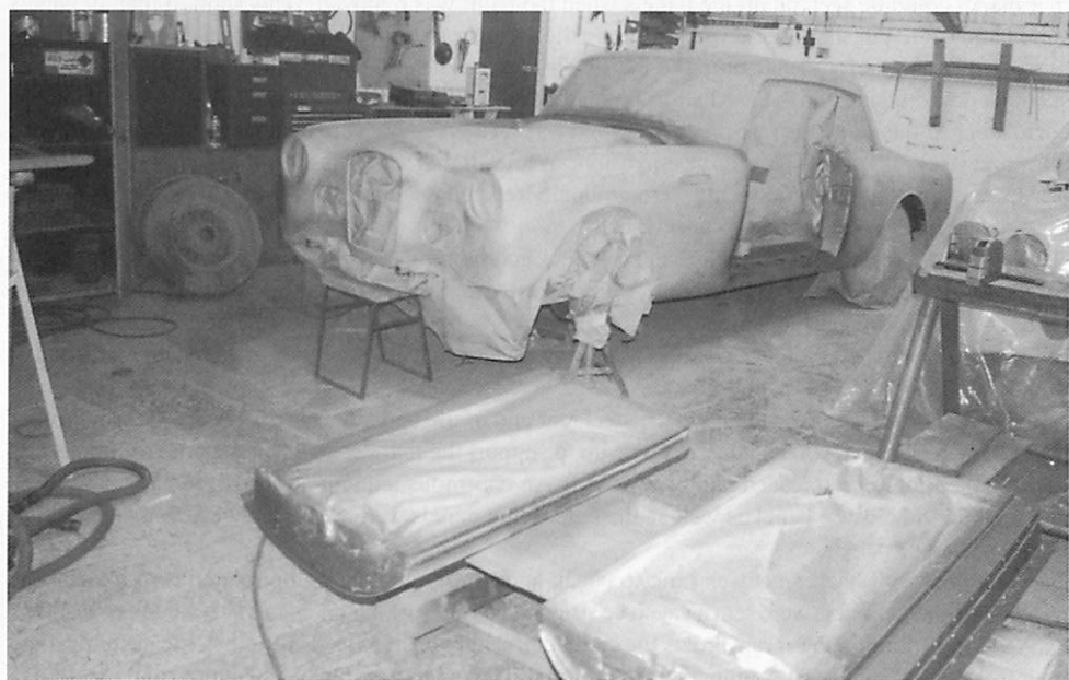
Before we knew it, the Millennium was upon us and there was still a lot to do. Profiling of the body surface was followed by priming and stopping. Here, the first stages of colour are being applied.
