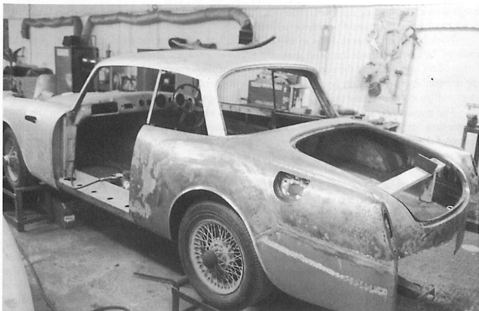
Roof back on, back panel partially cut away and installation of rear wing repair sections.
