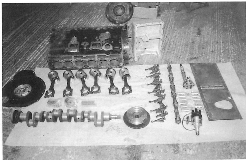
The engine was completely rebuilt, the electrical system rewired, converted to negative ground and electronic ignition installed.
