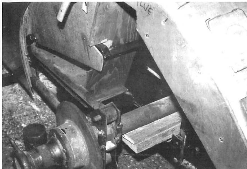
Trailing arms locating the rear axle (coil springs not shown)
