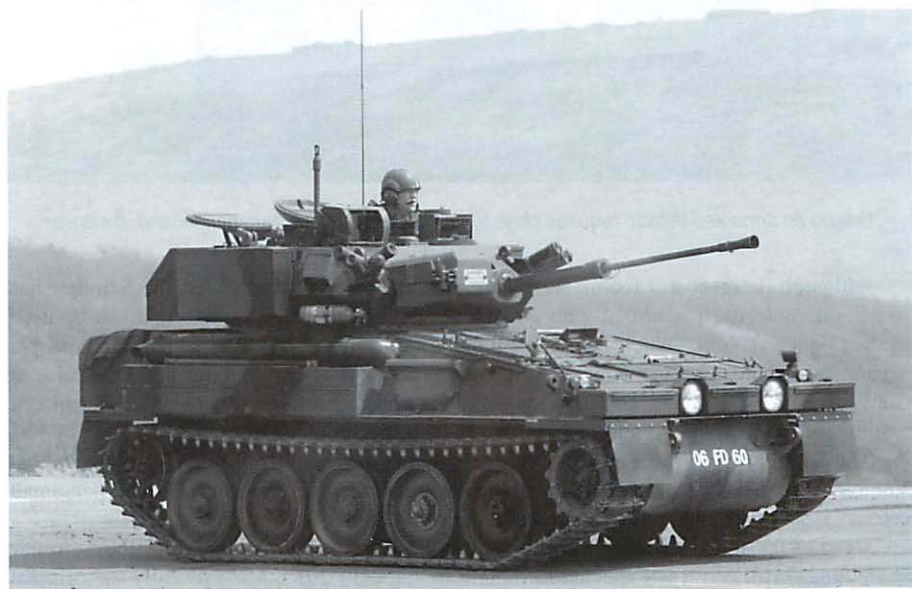
Although primarily a reconnaissance vehicle, the Scimitar is armed with cannon and machine gun
